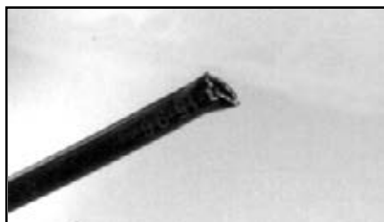
Bad cut - flattened
