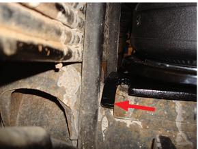
The tabs in the lower bracket shown in position under the jounce bumper strike plate.
