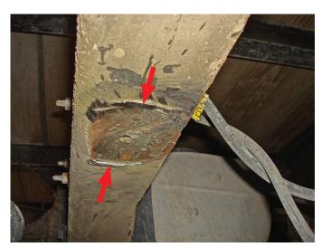
Grind remaining weld flush to the frame flange.
