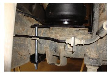
Right (passenger) side lower bracket installation
