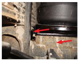
Lower bracket tab inserted under jounce bumper strike plate that is welded onto the axle.
