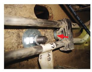
4 X 5/16" washers (P) stacked up behind line holder's in the front and in the rear of axle.
