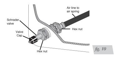
approximately 1/2" - to easily apply a pressure gauge or an air chuck (Fig. 10).
