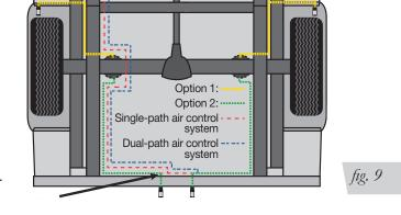
Whatever the chosen location, make sure there is enough clearance around the inflation valves for an air chuck.
