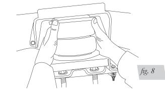
Maintain at least a thumb's width of clearance between the air spring and frame when uninflated.
