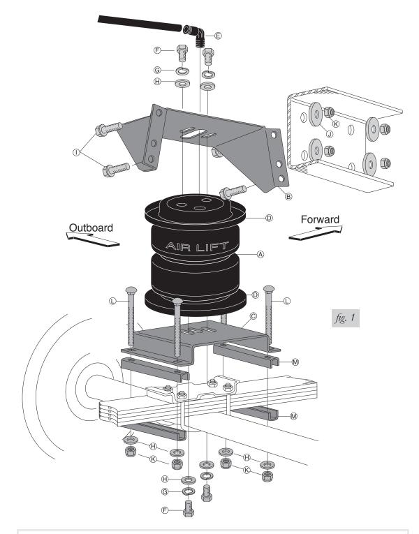
IMPORTANT: Check both sides of the frame rail for any interference or obstructions (specifically, propane lines) that may prevent install the air springs on the outside of the frame rail. If obstructions are present, use kit 57131, which mounts under the frame to the axle.
