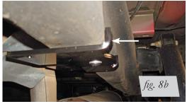
Passenger's side: Push bracket against frame and torque to 38 lb.-ft. (52Nm).
