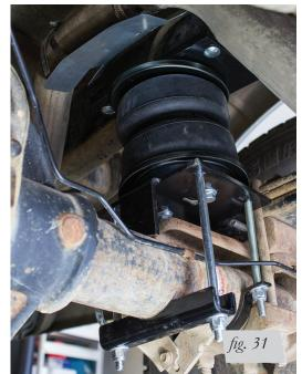
Right (passenger's) side: rear view of installation.
