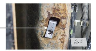
5. **All years**: On the passenger's (right) side, there is an emergency brake cable holder that is bolted on to a bracket welded to the axle with a self-tapping bolt. In order to make clearance for the axle strap, it will be necessary to cut this off or grind this bolt flush to the bracket (Fig. 6).
