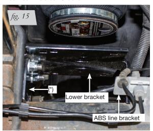
Driver's (left) side, rear view: Set the lower bracket into position on the axle making sure the inside leg is outboard of the ABS line bracket.
