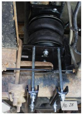
Left (driver's) side: rear view of installation.
