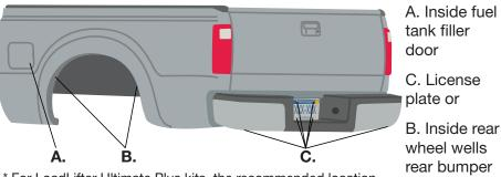
\* For LoadLifter Ultimate Plus kits, the recommended location for the Schrader valves is the rear bumper area or license plate.
