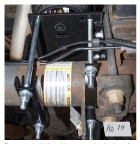
Passenger's (right ) side rearward axle view of finished installation torqued to 10 lb.-ft. (14Nm). finished installation torqued to 10 lb.-ft. (14Nm).
