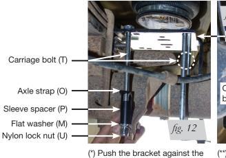
(\*) Push the bracket against the leaf spring in between the stock U-bolts.
