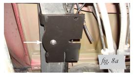
Driver's side: Push bracket against frame and torque to 38 lb.-ft. (52Nm).
