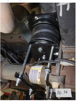
Right (passenger's) side: front view of installation.
