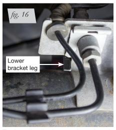
The lower bracket leg must be outboard (leaf spring side) of the ABS line bracket.
