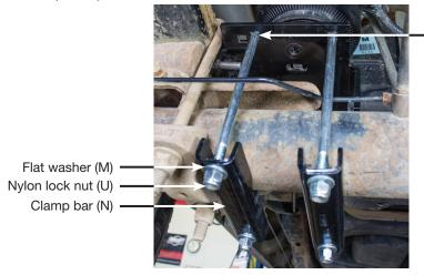
Driver's (left) side: The inside square holes must be used for the carriage bolts.
