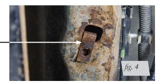
4. For the early 2004-08 models, install a new universal nut (V) into the large hole so that the threaded portion is up inside the frame (Fig. 5).
