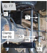
(\*\*) Passenger's (right) view towards the rear: Use outside set of square holes for carriage bolt (Q).
