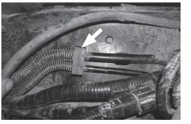
If equipped, this emissions/fuel line retaining clip must be pulled away from the frame in order to install the upper frame brace (D).
