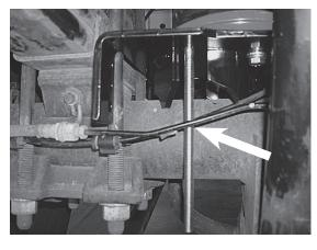
The long carriage bolt must go in between the axle and the hard brake/ ABS line on the driver's side.
