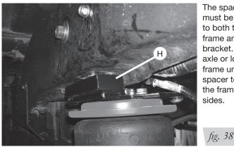
The spacer (H) must be parallel to both the frame and upper bracket. Raise axle or lower frame until the spacer touches the frame on both sides.
