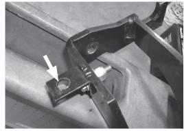
*fig.* 10 Attach the L-bracket to the brace in the position previously found using the hardware specified.
