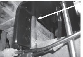
Rotate the lower bracket on the spring perch if necessary and push the bracket up against the U-bolts to put the lower bracket into position.
