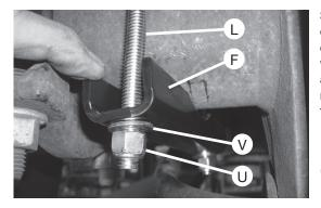
Set the clamp bar over the 3/8"-16 x 7" carriage bolts and cap with 3/8" flat washers and 3/8" nylon lock nuts. Leave loose at this time.
