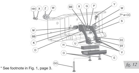
Attach the bracket to the frame using the 8 mm hardware noted.
