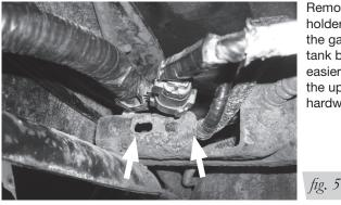
Remove the line holders from the gas/urea tank bracket for easier access to the upper brace hardware.
