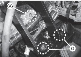
Raise the axle up while aligning the 3/8"-16 x 2" carriage bolt through the frame and the two 3/8"-16 X 1.25" carriage bolts in the upper bracket, through
