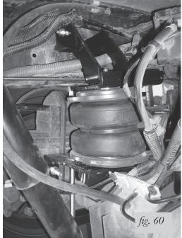
Left (driver's side) view of the kit installed from rear center of vehicle.
