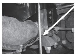
The long carriage bolt goes on the outside (backside) of the hard brake/ ABS line on the passenger's side.
