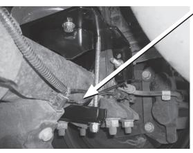
, It may be necessary on some models to not tighten the axle clamp bar evenly on the right (passenger's) side so that the clamp bar will clear the hard brake line.
