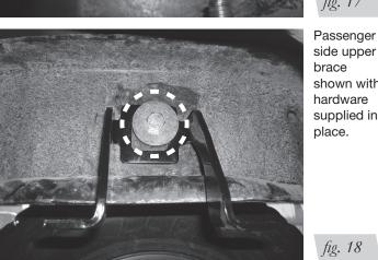
brace hardware, make sure frame (see Step 2). Note: The 1/2" thick washer (R) is not a half inch thick. It has a 1/2" hole and is a thick washer.
