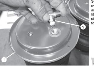
Set roll plate (I) over the bellows and install the fitting (Y) as stated. Repeat for both bellows.
