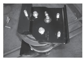
Spacer (H) set on bracket in position. The wide side of the spacer faces the outside of the vehicle.
