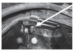
Insert the line holder previously removed into the L-bracket installed on the upper brace as shown.
