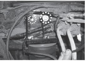
Tighten the 8 mm and 1/2" (or 3/4" from the existing fifth-wheel hitch) hardware securely. Repeat for the hardware on the opposite side.
