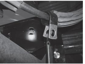
Set P-clamp over the emergency brake cable.
