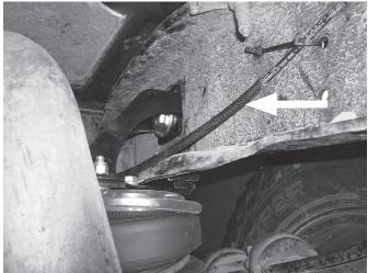
Hose heat shield shown in place on the right side (passenger) of the vehicle. Make sure heat shield is pushed up against the fitting once the hose is installed.
