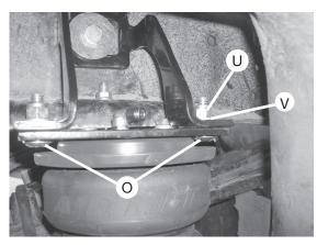
Cap the 3/8"-16 x 1.25" carriage bolts with 3/8" nylon lock nuts and torque to 15 lb.-ft. Repeat for both sides.
