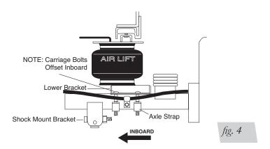
9. Align the air spring. With the unit aligned, tighten the lower bracket securely to the axle.
