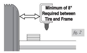
**NORMAL RIDE HEIGHT:** Normal ride height (no load) is defined as the distance between the bottom edge of the wheelwell to the center point of the hub with the vehicle in an "as delivered condition" (without a load, i.e. tool box, camper, etc.). Measurements should be taken before beginning the installation. The distance from the bottom edge of the wheel well to the center point of the hub should be recorded. All Air Lift kits are designed to be installed and operated at normal ride height.
