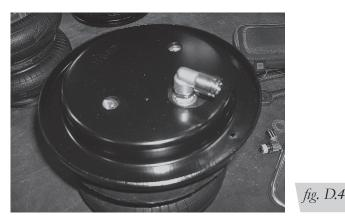
2. Flip the assembly over and set a roll plate (D) on the bottom of the air spring. Install the lower bracket onto the assembly, making sure the flange of the lower bracket is on the fitting side of the air spring assembly. Attach the lower bracket with two 3/8"-24 x 7/8" hex cap screws (E), 3/8" lock washers (F) and 3/8" flat washers (G) (Fig. D.5). Torque the mounting hardware to no more than 20 lb.-ft. (27 Nm).
