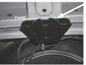
Bracket must be parallel with the frame before tightening.
