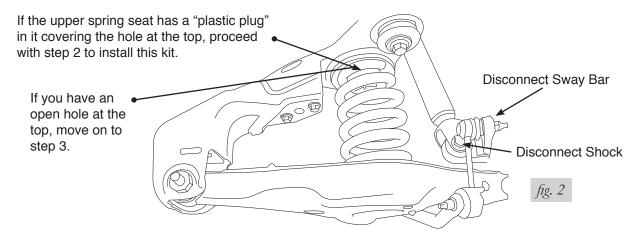
Almost all of these applications have a hole in the upper spring seat, if you have a "plastic plug" covering the hole in the upper spring seat, proceed with step 2. If you have an "open hole" in the spring seat that you can see, move on to step 3 for further instructions.
