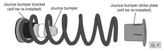
6. It will be necessary to enlarge the center hole in the upper jounce bumper bracket. Drill the existing hole out with a 1/2" drill bit (fig. 5).
