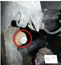
6. Attach the sensor wire to the shock (fig. 13). Torque bolt to 10 Nm (7 ft-lbs.).
