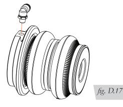
4. With the fitting on the top side, apply the air spring over the lower spring land and position the fitting in a desired location, free from air line routing obstructions (Figs. D.18 & D.19).
