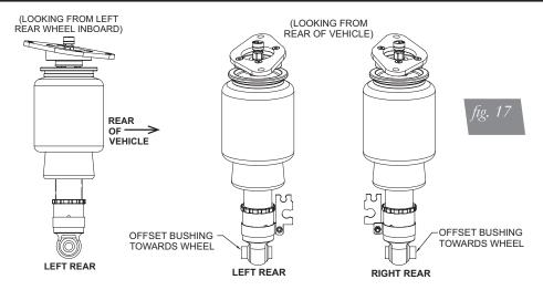
5. Align the lower eye mount with the longer bushing offset against the mounting surface. Install the lower bolt but do not torque at this time (Fig. 18). (Torque of the lower mount bolt should be done when the vehicle is at ride height.)
