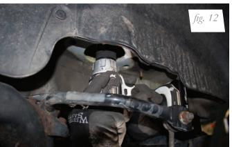
3. Install the leader line into the air spring. Apply thread sealant to the threads of the leader hose. Tighten the appropriate fitting to the air line (one and three-quarter turns beyond hand-tight). Tighten the leader line into the air spring (one and three-quarter turns beyond hand-tight) (Fig. 13).
