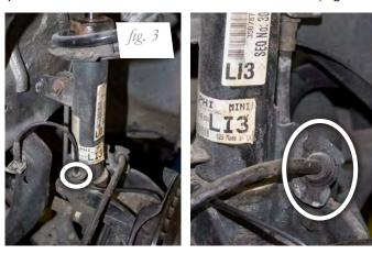
2. Unthread the stabilizer bar end link nuts from the strut and bar. Note orientation and placement of link. Remove the end link. (Fig. 5).
